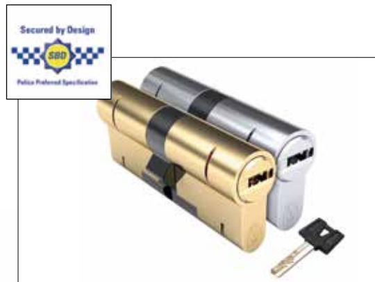
High Security Cylinder (optional extra) Superior physical strength - Cylinder design that prevents lock bumping Anti-snap now with break points allowing interior key to work even if external snap damage occurs
